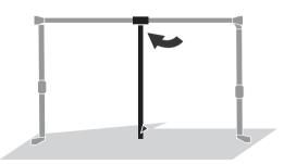
On windy days secure the line by looping the strap through orange block in centre of frame. Anchor the other side of the strap to ground using a tent peg, sandbag or weights.
