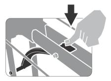
Lock legs in place by depressing tab ( do this on both sides )
