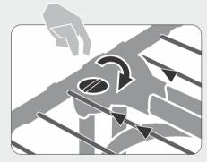
Step 4) Turn ratchet clockwise to remove slack from line 5 (DO NOT over tighten).
